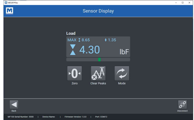
▲ View real-time, peak, and average load data, and zero (tare) and clear peaks.
