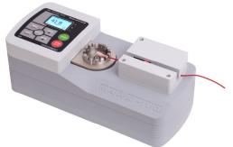
Thank you for purchasing a Mark-10 WT3-201M wire crimp pull tester, designed for pull test applications up to 200 lbF (1,000 N).
