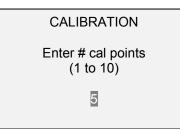
The tester can be calibrated at up to 10 points. Enter the number of calibration points (at least one point must be selected).
