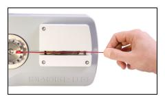
3. Note the protective red safety guard (circled, below), which automatically rotates into position as the cam mechanism closes.
