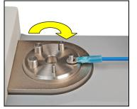
2. Insert the loose end of the wire between the cams in the mechanism. Keep the wire taut as it is inserted. If auto-start is enabled, the test will begin when the switch is activated (refer to later sections for operational details). Refer to the image below:
