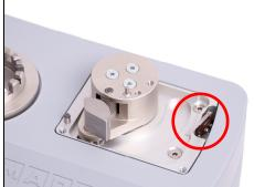
Use a small brush to collect and remove debris. To avoid possible damage to tester components, **DO NOT** use compressed air.
