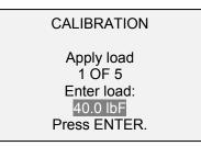
Use the **UP** and **DOWN** keys to adjust the load value as required. The load values default to evenly spaced increments, as indicated by the previously entered number of data points. Apply the calibration load. Then press **ENTER**.
