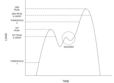
**11.3 Auto Output Settings** Select the output type. Select RS-232/USB and/or Mitutoyo outputs, and select First and/or Second peaks. The display will appear as follows:
