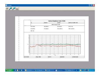
DataView software for TR200/220 works with surface roughness tester TR-200 and TR-220 for managing, analyzing, printing and searching measured data and graphs. This software is designed to complete all the operation without touch any key of TR-200/220. With the software you can see the profile graph more clearly and expediently and store data of many measurement onto your PC.
